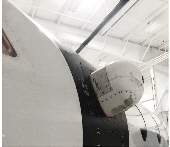
Figure 6. A) Hemisphere configuration mounted in AAOL-BC aircraft. B) Hemisphere on full cylinder configuration mounted on AAOL-BC aircraft.
