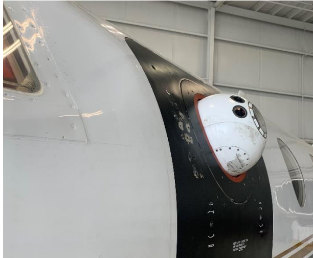
Figure 6. A) Hemisphere configuration mounted in AAOL-BC aircraft. B) Hemisphere on full cylinder configuration mounted on AAOL-BC aircraft.
